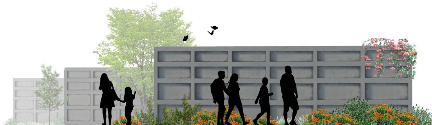
GATES As part of restoration, the mechanical elements of the spillway will be removed. The large gates that are used to regulate the levels of the reservoir are repurposed as a sculptural element. A footpath and native meadow flow through passages between the gates on the way to the river.
